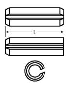
Both ends are chamfered on pins less than 10 mm in diameter; only one end may be chamfered on 10 mm and larger diameter pins. Measure length from end to end. ISO 8752 is similar to DIN 1481. Also known as Roll Pins. Mounting hole nominal diameter tolerance zone is H12.
