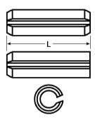
Both ends are chamfered on pins less than 10 mm in diameter; only one end may be chamfered on 10 mm and larger diameter pins. Measure length from end to end. ISO 13337 is similar to DIN 7346. Also known as Roll Pins. Mounting hole nominal diameter tolerance zone is H12.
